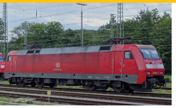
In the early 1990s, a need for modern three-phase AC locomotives for freight transportation became apparent. This resulted in a DB tender for the development of such a vehicle in 1993. The Siemens/Krauss-Maffei consortium was able to win the contract and the prototype 152 001-4 was built by 1995 based on the experience gained with the 127 001-6 test vehicle.
